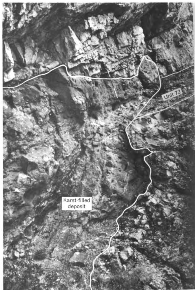
FIGURE 10.—Karst-filled deposit in the upper member of the Mission Canyon Limestone in the SE¼ sec. 35, T. 2 S., R. 9 E. Note the crosscutting relation of the karst-filled deposit to the siltstone (unit 72). Base of stadia rod (painted in 1-ft intervals) is 47 feet below top of the upper member.
